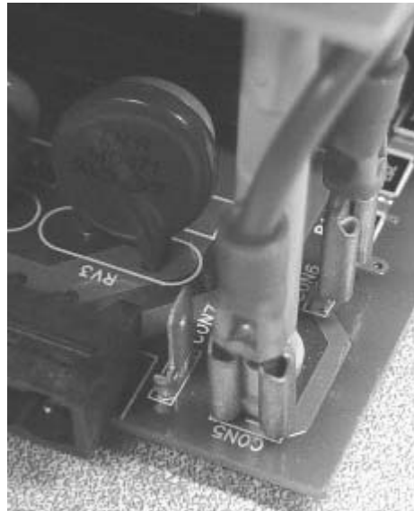
Grounded Input Power Configuration (Factory Default) CON5 Jumped to CON6
