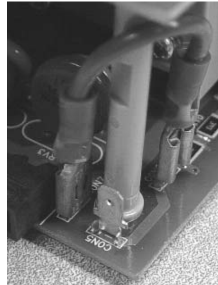
Ungrounded Input Power Configuration (Field Selected) CON6 Jumped to CON7
