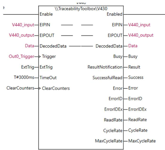
The Traceability Toolbox Sysmac library complements this framework by providing essential data capture building blocks. These blocks facilitate the effortless creation of retrofit data collection systems using Omron data capture devices from Sysmac Studio.
