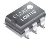
**Dual Independent Single Pole Normally Closed: 1-Form-B** - Operational temperature range of -40° to 85°C
